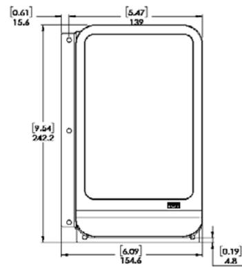
Figure 6 Front view with bracket
