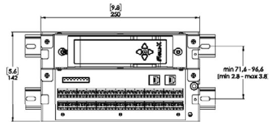
Figure 1 Horizontal DIN rail mount
